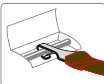
F. Pull the tether strap on another end back to tighten the top tether.
