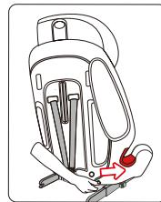
B. Loose the harness strap and pull strap out off the strap yoke as shown in right picture.
