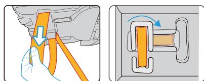
E. Remove the 5-point harness system then remove the headrest cover and the shell cover.
