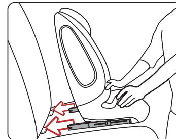
C. Grasp the seat body to check the seat if it is fastened tightly or shakes. If the seat shakes and the ISOFIX connectors are pulled out, please repeat the above steps and install it again.
