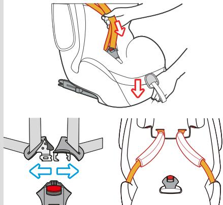
C. The correct belt height of the shoulder pads is attained when the strap disappears into the shell slightly above the shoulder of the child.
