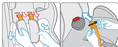
D. After above steps, draw whole strap out from the bottom of seat. Rotate buckle clip to the shown position, then take it out from seat base.
